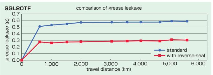
Reverse-seal makes a "Grease Pocket" between the two seals that realizes MAINTENANCE FREE by reducing grease leakage and loss.
